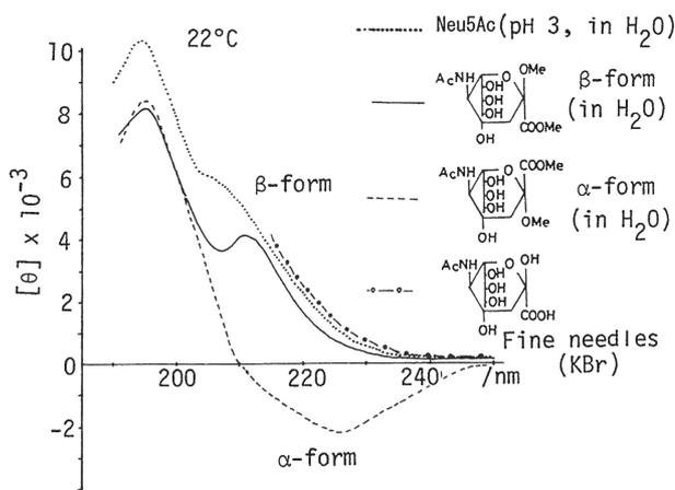
Fig. 39. CD spectra of sialic acids Neu5Ac and its  $\alpha$ - and  $\beta$ -methyl glycosides.
