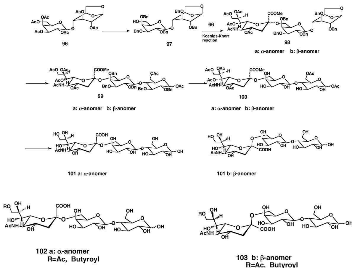
Fig. 28. Synthesis of Neu5Ac(2→6)lactose and 9-*O*-acyl derivatives.
